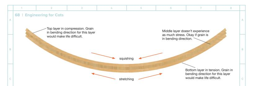
When the wood is bent as shown (see above), the top layer will want to get shorter (loaded in compression), the bottom layer will want to get longer (loaded in tension), and the middle layer won't change much. To allow the wood to bend, the grain should be running side to side. If the grain is in the bending direction, the wood will build up larger internal stresses when bent. This could lead to cracking, screws popping out, and increased frustration.
